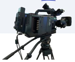
The Vislink INCAM GV 5G is a fully integrated HEVC 4K UHD, HDR-ready wireless video transmitter and receiver, designed for use with Grass Valley's LDX 100 Series live production cameras. The INCAM GV 5G leverages the capabilities of private 5G cells in studios and stadiums, as well as public sliced 5G networks. It complements the latest design enhancements incorporated into the Grass Valley LDX 100 Series cameras for heightened usability and ergonomic operation.
